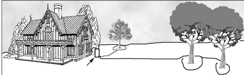
A 55 gallon drum is shown above collecting water from a washing machine or sink drains. The drum may be located in a basement for year-round use and regularly pumped to the outdoor mulch basins around the trees. The hose is perforated only around the trees, where it is buried in a shallow trench under a heavy mulch. Entire length of hose may be buried for frost protection.
